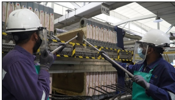
[TES workers scratching graphite from waste batteries from press filters]
